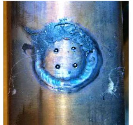
Figure 3.4: A picture of a thermocouple disc.
