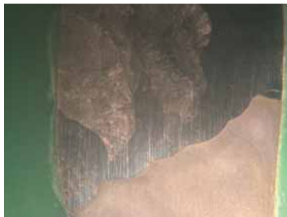
Figure 19, overview of sample 6 with etched weld metal (2x)
