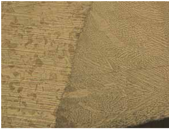
Figure 23, in the root of sample 3, transition from stainless steel to weld metal (5x)
