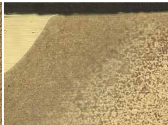
Figure 26, in the top of sample 5, HAZ on the low alloyed steel side (5x)
