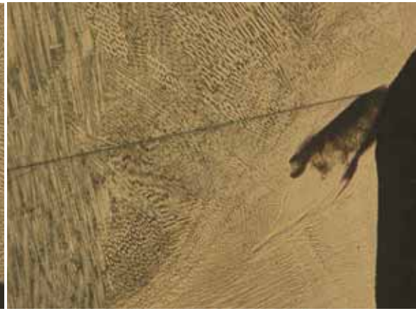
Figure 24, in the root of sample 3, part of low alloyed steel that is not dissolved in the weld metal (10x)
