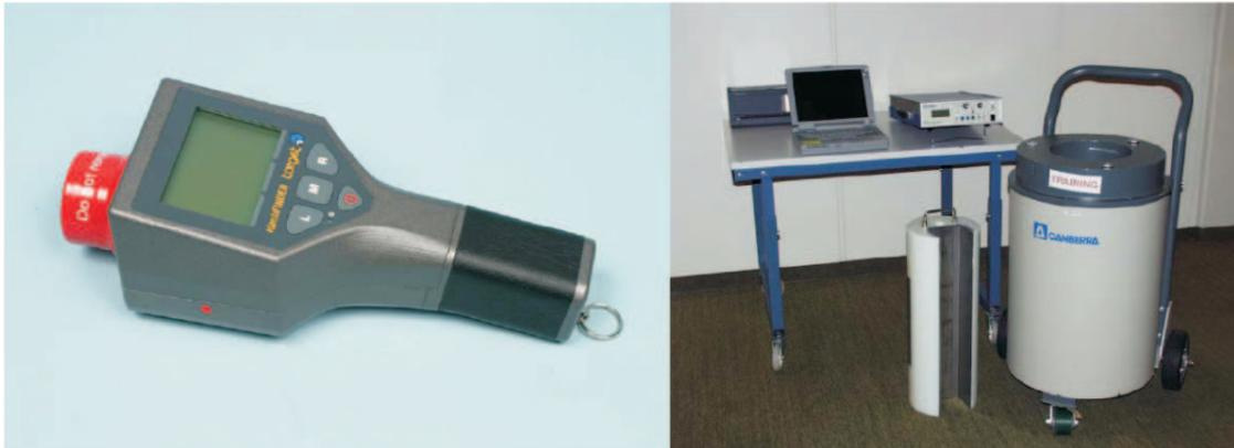
**Figure 3.1:** The handheld HM-5 (right) shown together with an active well neutron counter (left).
