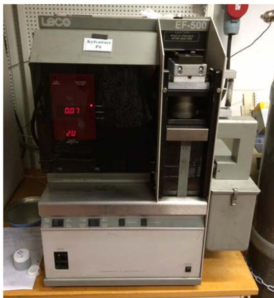
Figure 2.5: LECO TC-136 inert fusion gas instrument.
