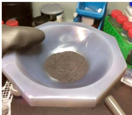
Figure 4.5: Resulting uranium nitride powder.
