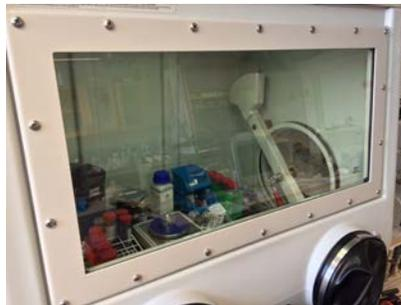
Figure 5.1: Glove box used for mixing powders.
