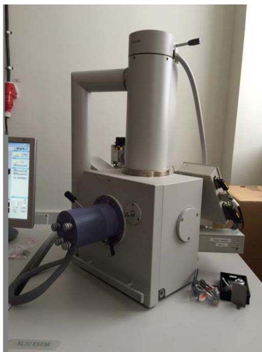
Figure 2.2: XL-30 field emission ESEM microscope.
