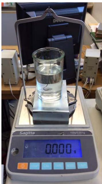
Figure 2.1: Setup used for density measurement.
