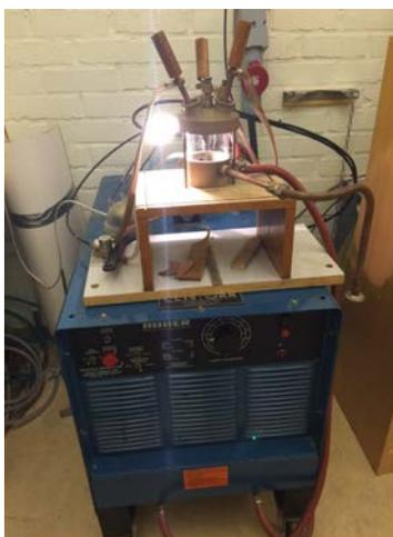
Figure 3.2: Triple arc melter used for melting alloys.
