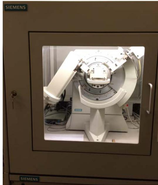
Figure 2.3: Siemens D5000 x-ray diffractometer.
