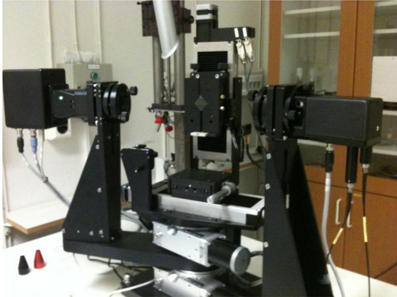
Figure 8: Spectroscopic ellipsometer at Linköping University
