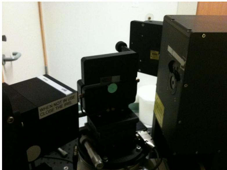
Figure 9: IR-ellipsometer at Linköping University
