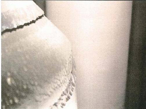
Figure 1: Corrosion on the welding of Alloy 82 at a CRDM-nozzle. [14]
