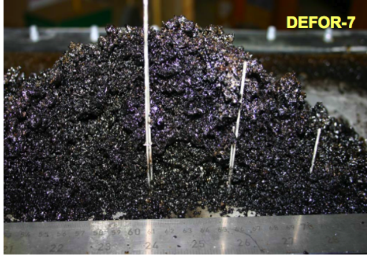
Figure 1.1: Picture from DEFOR experiment, showing high porosity and different internal cooling channels in the debris bed, printed with permission from T. N. Dinh.
