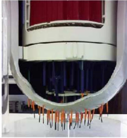
**Figure 3.2:** This model shows the in-core instrumentation tubes in the bottom of the core where the detectors are inserted.
