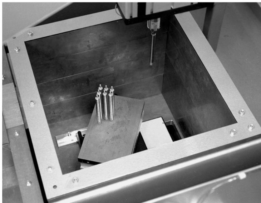
**Figure 5.3.** The laboratory device. A robot with three axes (above) can place the rods of the fuel model in different configurations on a magnetic table (below). A part of the collimator-detector package is seen to the left in the photograph below.
