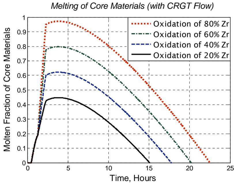
Figure 1.2: Molten fraction of core materials in a reference BWR with different mass of Zr oxidized. CRGT cooling flow rate is 15 kg/(m<sup>2</sup>.sec) activated from the accident start.
