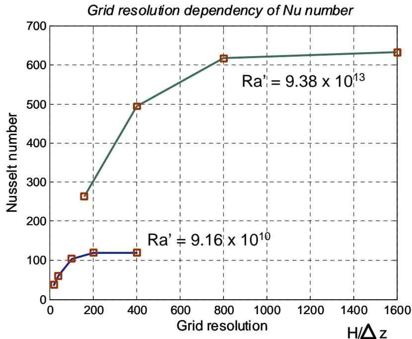
Figure 3.2: Grid resolution dependence of heat transfer coefficients.
