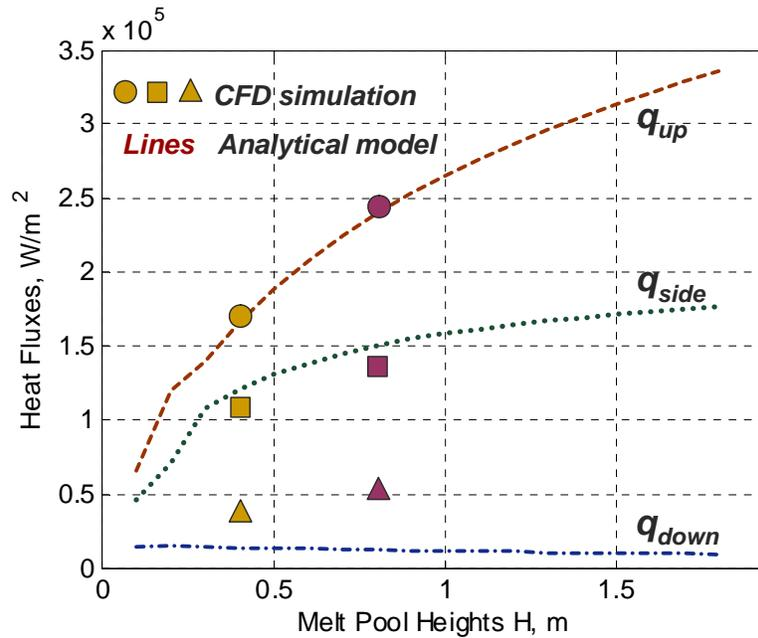
Figure 3.4: Analytical model and CFD simulation energy splitting.
