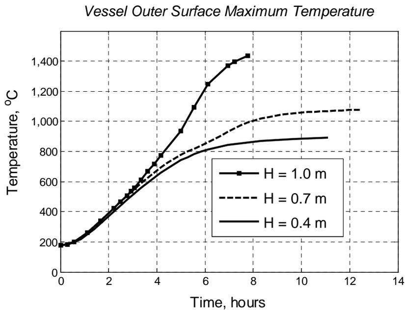
Figure 6.4: Evolution of vessel wall maximum temperature.
