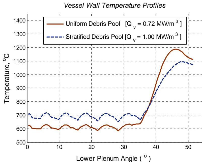
Figure 6.7: Temperature profiles of the vessel external surface.
