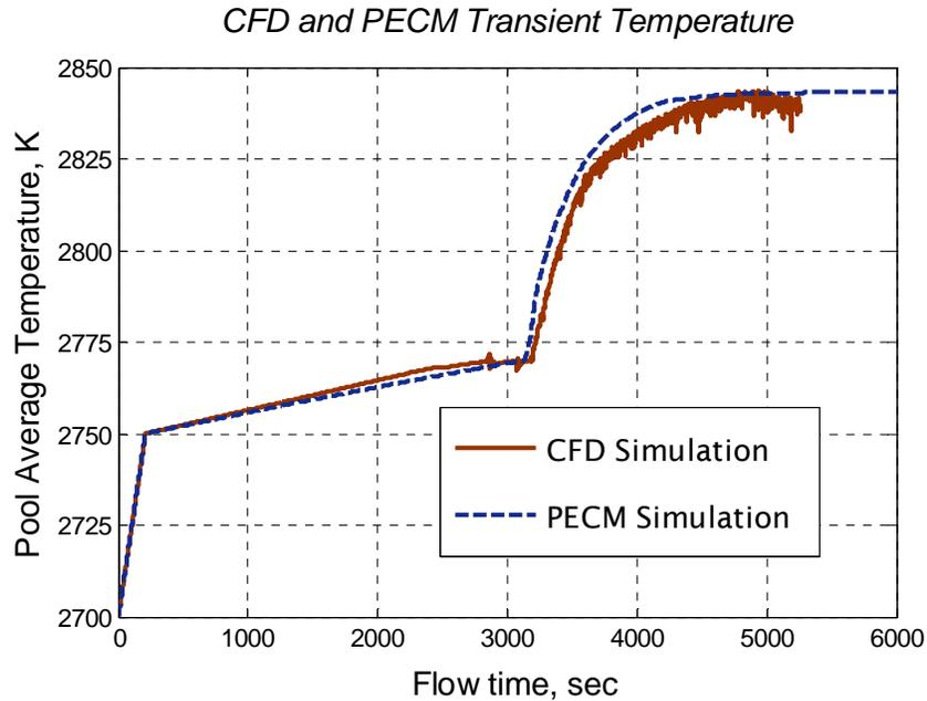
Figure 5.2: CFD and PECM transient melt pool temperatures.
