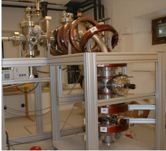
Left: The pulsed positron beam at Chalmers University of Technology. The positron timing is measured by a multi channel plate positioned at the end of the beam line, at the bottom of the picture. Right: Time spectrum recorded with both chopper and buncher operating at 50 MHz, and positron energy is 250 eV. The width of the positron pulse is about 0.5 ns.
