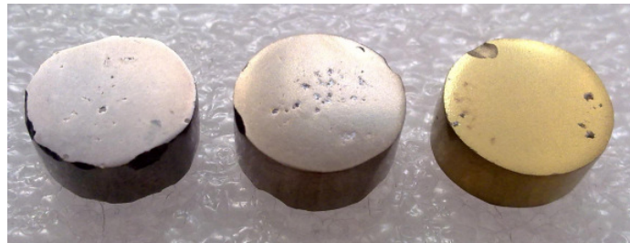
Figure 2: SPS sintered pellets, from left to right; UN pellet, (U,Zr)N pellet, ZrN pellet
