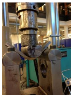
Fig.5. Material testing of weld, from thesis by Hanna Johansson
