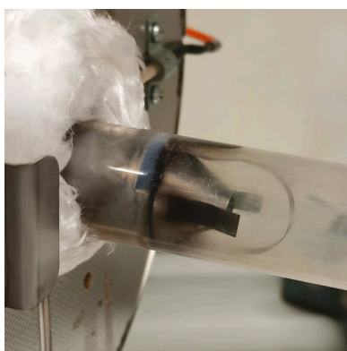
Figure 2.17: Ta funnel made from metal sheet.
