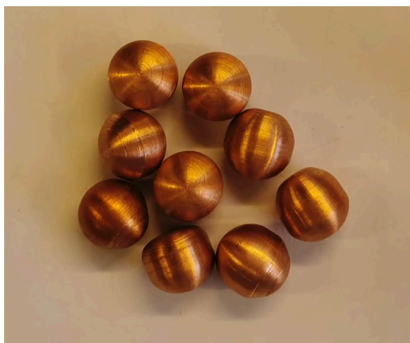
Figure 2.12: The nine copper balls used for mixing and crushing.
