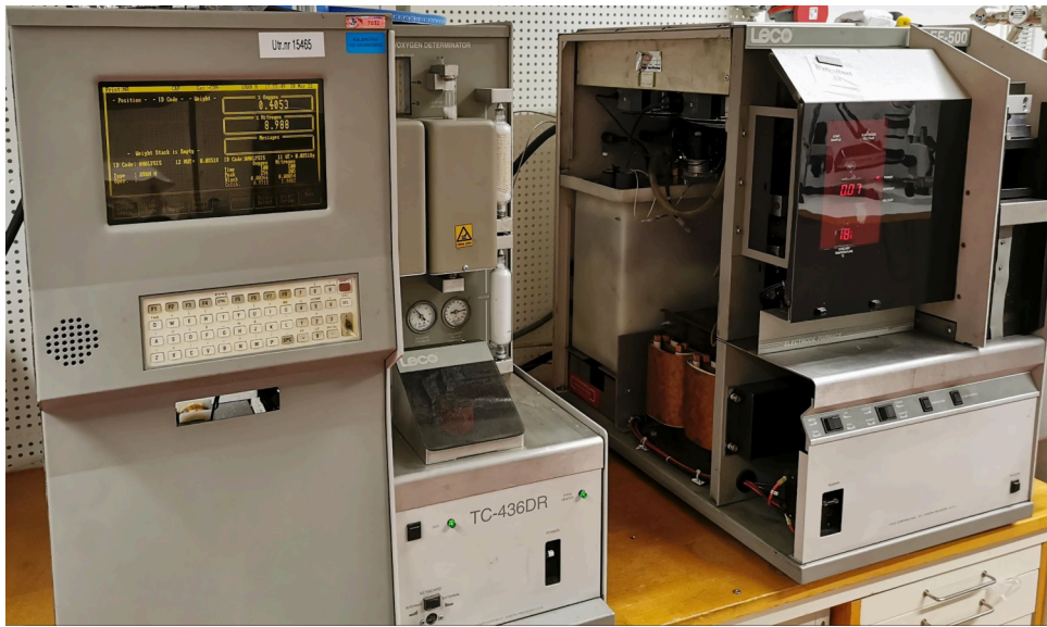
Figure 2.5: The LECO EF-500 oxygen/nitrogen analyzer.
