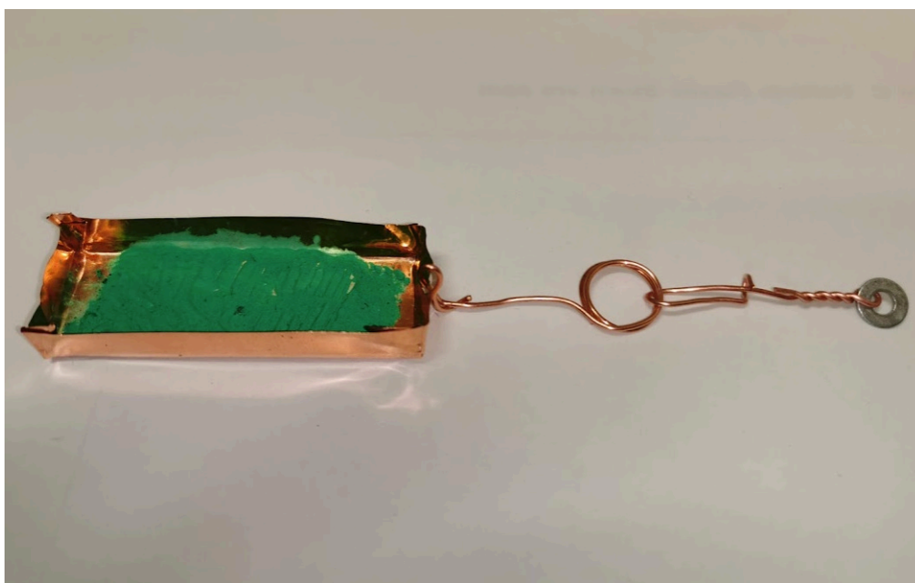
Figure 2.10: The magnetic retractable loaded Cu boat
