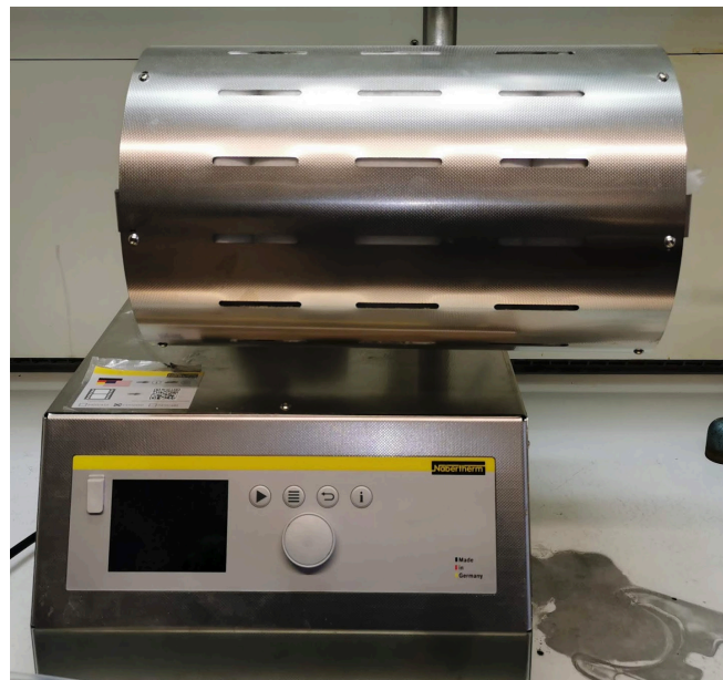
Figure 2.6: Nabertherm RT 50-250/13 tube furnace.
