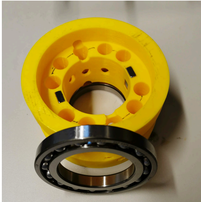
Figure 2.21: The 3D-printed pulley with a ball-bearing and the magnets attached.
