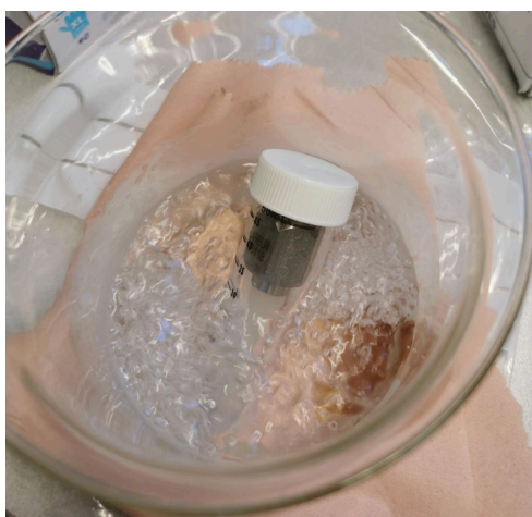
Figure 2.1: The \text{UF}_6 canister in a tube submerged in a liquid nitrogen bath.
