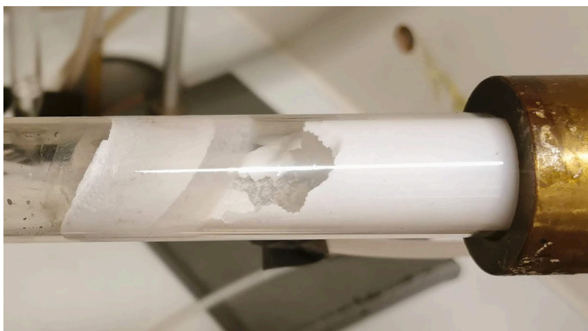
Figure 3.1: The slightly deformed NH 4 F layer at the end of the run.
