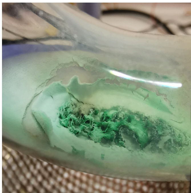
Figure 4.2: The green reaction product after exposure of UF 6 to NH 3 gas.
