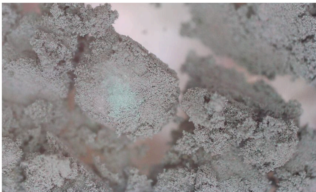
Figure 3.5: Microscope image of the unreacted UF 4 in the sample.
