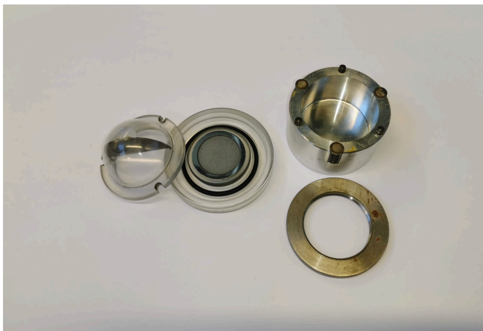
Figure 2.3: The BRUKER airtight sample holder with the assembly tool.
