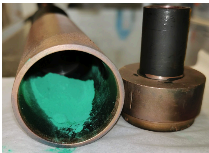
Figure 3.13: The upscaled drum loaded with UF_4 .
