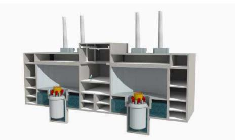
Figure 2.2: Layout of twin SEALER-UK units positioned underground [Published with permission from LeadCold]
