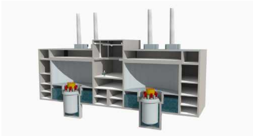
Figure 3.1: A cross sectional view of the reactor building in a proposed SEALER-UK nuclear power plant. Published with permission from LeadCold.
