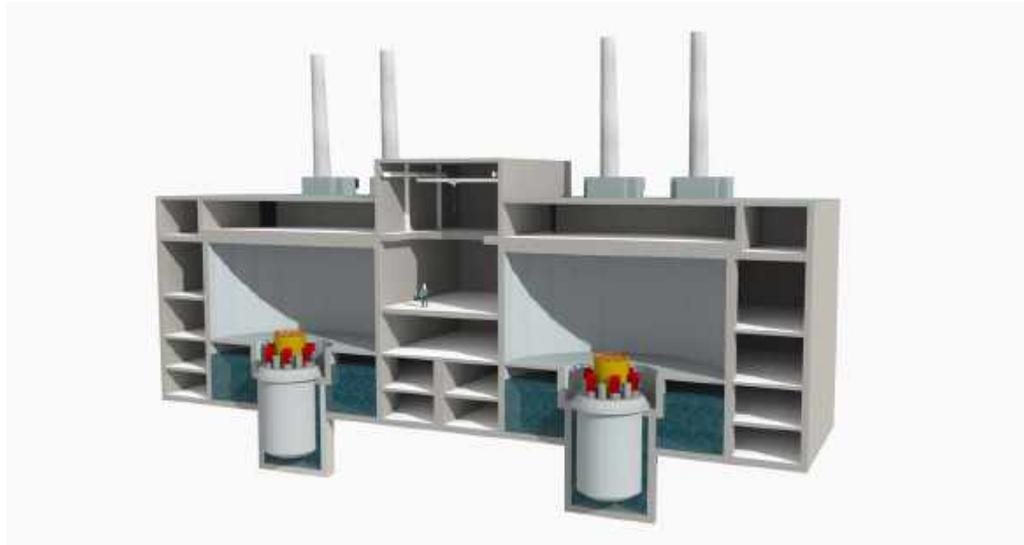
Figure 2.2: Layout of twin SEALER-UK units positioned underground [Published with permission from LeadCold]
